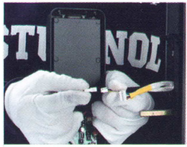
5. Connect the power cord of the front lock and the cat's eye line
