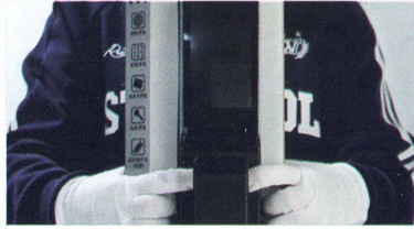
10. Press and hold the "on/off key" of the rear lock at the same time until the prompt sound sounds, and press the "#" key on the front lock to restore the initialization, and the installation is complete
